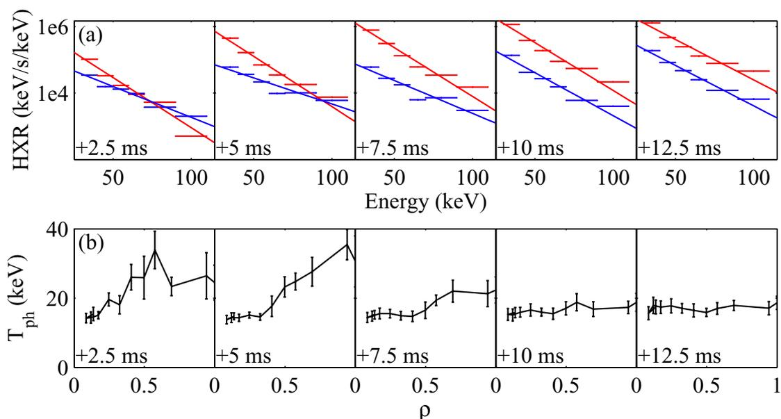
**Fig. 2** (a) HXR emissivity as a function of energy in 5 snapshots after the ECCD switch-on ( $t=0$ ), for a central (red) and an off-axis (blue,  $\rho \sim 0.6$ ) chord; (b) spatial profiles of the photon temperature for the same snapshots ( $\rho$  here indicates the minimum normalised radius for each chord, i.e. the point of tangency to the flux surface).
