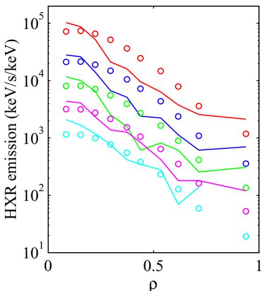
**Fig. 3** (a) Predicted (lines) and measured (circles) HXR emission as a function of chordal spatial location for 5 energy channels of 8 keV width in the 16-56 keV range (descending amplitude for increasing energy).
