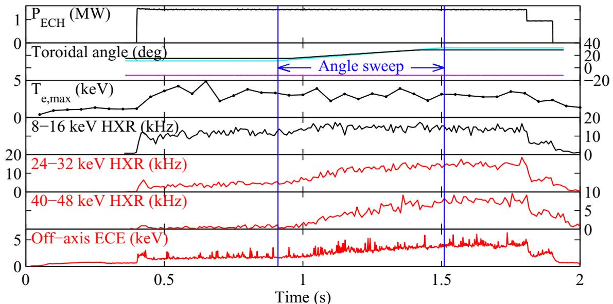
**Fig. 1** Sweep of the EC toroidal injection angle on two out of three launchers: the traces shown are the total EC power, the toroidal angles of the three launchers, the peak electron temperature, three energy channels of the HXR signal on a central chord and an off-axis ECE signal.
