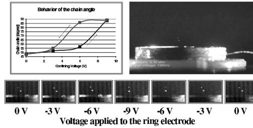
FIGURE 2. Experiment: levitation of two particles.
