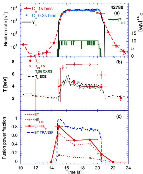
Fig. 2 MPR results for discharge #42780 on the time evolution of count rate  $C_n$  (a), temperatures (b), and fusion power fractions (c) compared with other data
