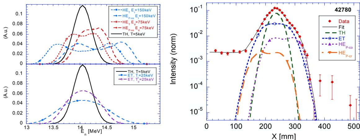
Fig. 1. Spectral components (left panel) used to describe the neutron emission from NB plasmas and applied in the analysis of MPR data for JET discharge #42780 (right panel).
