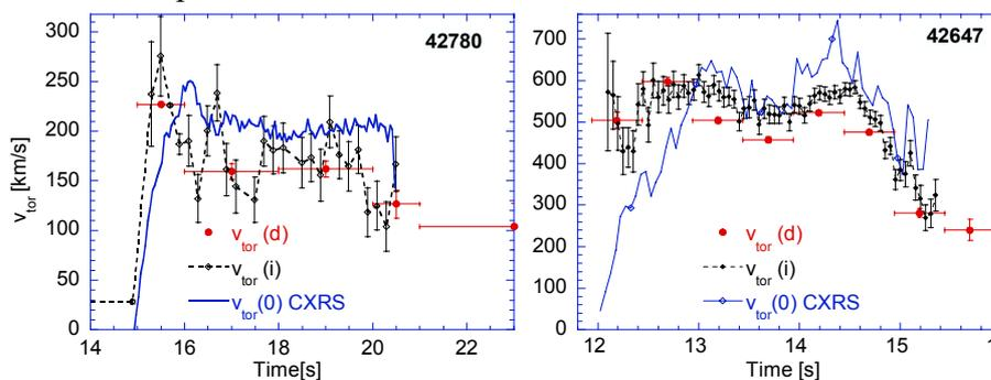
Fig. 3 Inclusive and detailed study of toroidal rotation as compared with CXRS data for #42780 heated with NB( $T^\circ$ ) (left) and #42647 heated with NB( $D^\circ, T^\circ$ ) (right).
