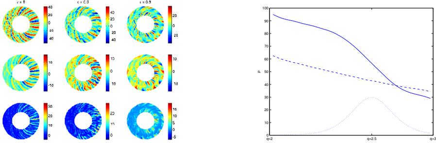
FIG. 1: (Left) Contour plots for electrostatic potential fluctuations, in the poloidal plane for three values of shear ( $\epsilon = 0, 0.3, 0.9$ ). (Right) Equilibrium pressure profile for the shearless case (dashed line) and strong rotation shear (solid line). Dotted lines stands for the radial profile of the shear flow
