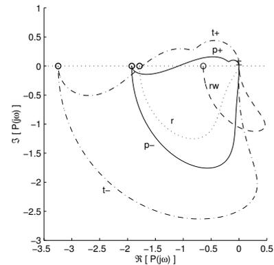
Figure 1: Nyquist plots of open loop transfer function for radial sensors, small (dotted) and wide (dashed), internal and external poloidal (solid) and toroidal (dash-dotted) sensors.
