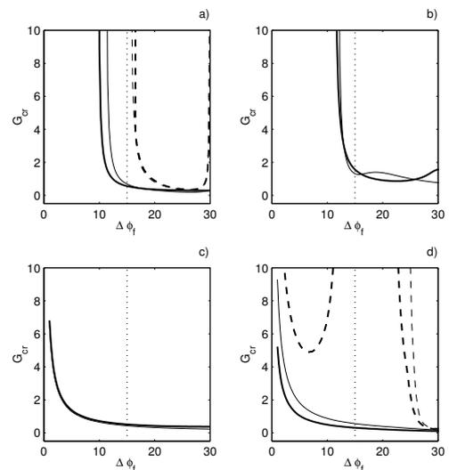
Figure 2: Minimum (solid line) and maximum (dashed line) gain  $K_{cr}$  necessary to stabilise all the modes, as function of the toroidal width of the coils, for (a) radial small, (b) radial wide, (c) poloidal internal, (d) toroidal internal sensors. Bold lines refer to the equilibrium  $\Theta = 1.58$  and normal lines to  $\Theta = 2.07$ .
