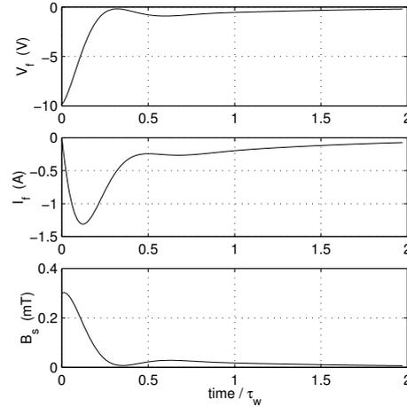
Figure 3: Time evolution of the feedback voltage  $V_f$ , current  $I_f$  in the coil and magnetic field perturbation  $B_s$  at the sensors. The time is normalised to the wall time.
