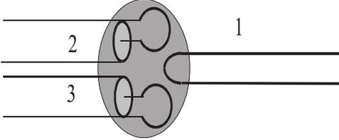
Fig.1. Quarter-wave resonator (1), exciting (2) and receiving (3) lines
