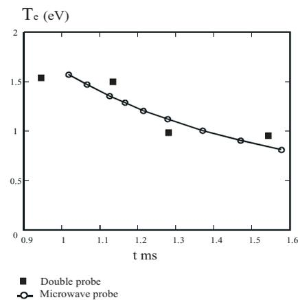
Fig.2. Results of measuring time dependence of the electron temperature obtained by means of a double probe and a microwave probe
