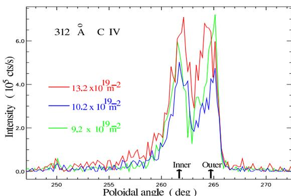
Figure 7. Poloidal scan of the 312Å, CIV line intensity for pulse 53982/57.5s (green), 53977/55.8s (blue) and 53983/57.5s (red) showing the C density dependence in He plasmas.
