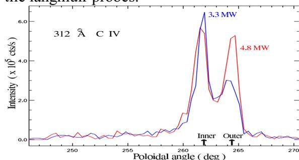
Figure 3. Poloidal scan of the 312Å, CIV line intensity for pulse 50420 at 58.8s (red) and 54.3s (blue) showing the power dependence in D plasmas.
