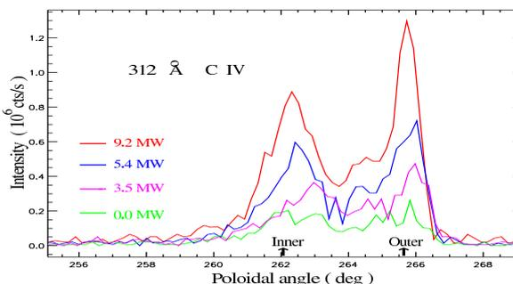
Figure 4. Poloidal scan of the 312Å, CIV line intensity for pulse 53977/57.6s (green), 53986/57s (magenta), 53982/57.5s (blue) and 53986/61s (red) showing the power dependence in He plasmas.
