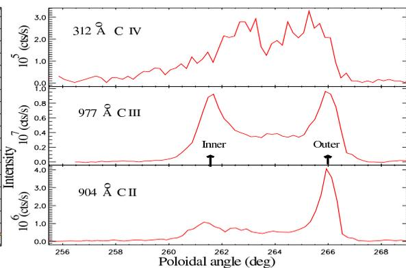
Figure 6. Poloidal scan of the 904Å CII, pulse 53980/57.6s, 977Å CIII, pulse 53978/57.5s and 312Å CIV line intensities, pulse 53986/55s, observed in He plasmas.
