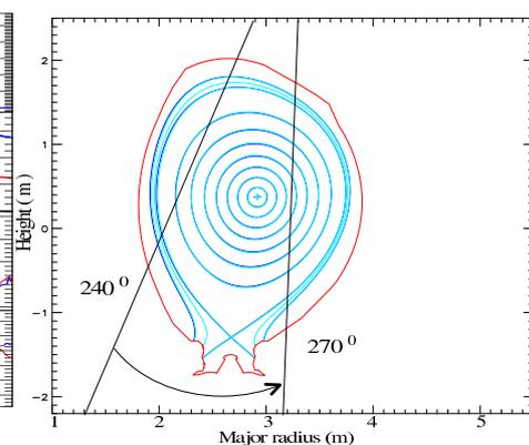
Figure 2. The magnetic configurations of pulses 50414 (D) and 53981 (He), also showing the extreme positions of the VUV spectrometer's poloidal scan.
