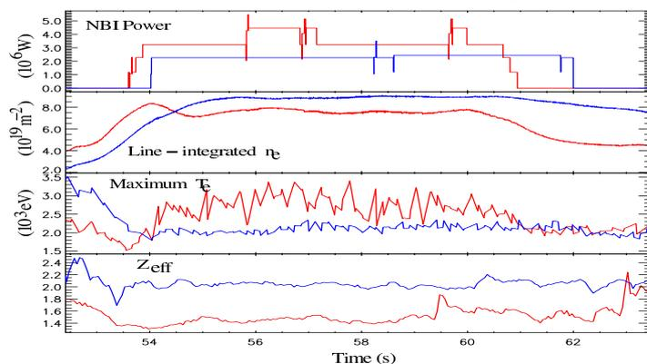
Figure 1. NBI power, line-integrated  $n_e$ , maximum  $T_e$  and  $Z_{eff}$  for D pulse 50414 (red) and He pulse 53981 (blue) used in the EDGE2D simulations.
