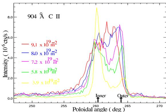
Figure 5. Poloidal scan of the 904Å, CII line intensity for pulse 52690 at 56s (yellow), 57s (green), 58s (magenta), 59s (blue) and 60s (red) showing the density dependence in D plasmas.
