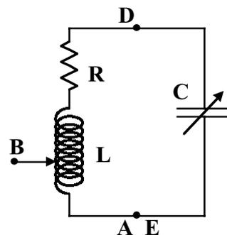
Fig.4 Equivalent circuit of the tunable strap.
