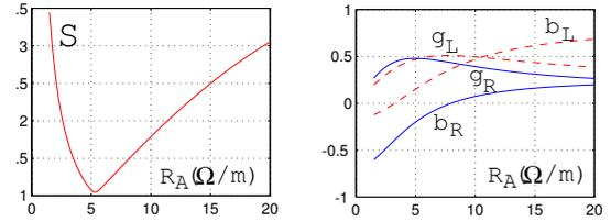
Fig.6 Matching characteristics of the symmetric excitation of the antenna pair ( $C_{pR} = 80.4$  pF,  $C_{pL} = 80.4$  pF,  $l_{BR-T}/\lambda = 1.285$ ,  $l_{BL-T}/\lambda = 1.855$ ,  $f = 32.5$  MHz)
