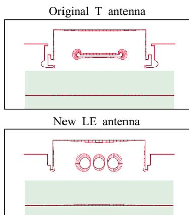
Fig.1 Cross-section of one antenna box of the "LE" and of the "L" antenna pairs with results of 2-D modelling.
