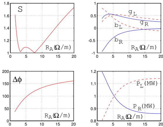
Fig.5 Performances of the optimised conjugated T operation ( $C_{pR} = 80.4$  pF,  $C_{pL} = 67.2$  pF,  $l_{BR-T}/\lambda = 1.248$ ,  $l_{BL-T}/\lambda = 1.717$ ,  $f = 32.5$  MHz)
