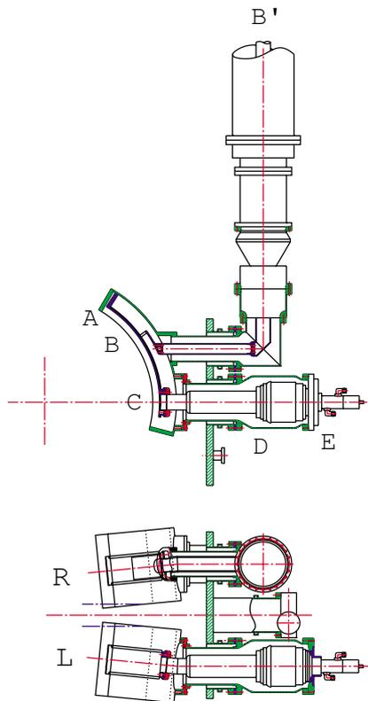
Fig.3 a), b) Side and top view of the tunable antenna pair. The top view shows on the R side the upper part and on the L side the lower part.
