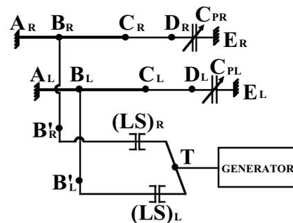
Fig.3c) Schematic diagram of the load insensitive antenna system
