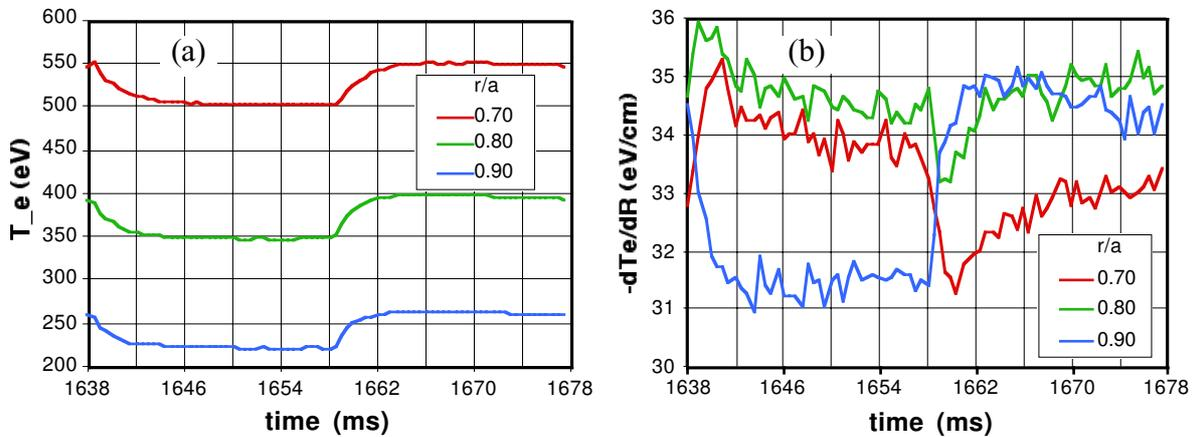
**Fig. 2. (a) Electron temperature and (b) radial gradient boxcar-averaged over 17 ECH periods. The ECH resonance is centered at  $r/a \approx 0.815$ .**
