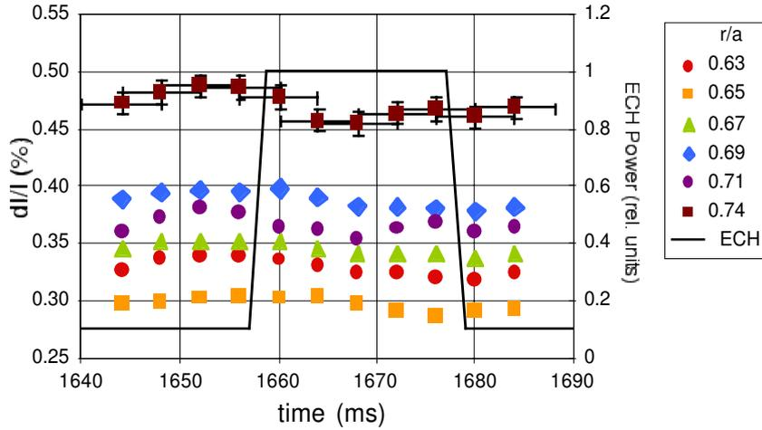
**Fig. 1. Emission-intensity fluctuation levels for the six BES poloidal arrays during an ECH cycle.**
