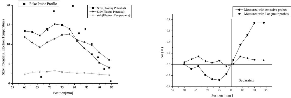
Fig. 3: Properties of the fluctuations of the plasma potential, the cold probe floating potential and of the electron temperature; (a) rms-values of  $\Phi$ ,  $V_{fl}$  and of  $T_e$ ; (b) correlation coefficient between  $\Phi$  and of  $T_e$ .
