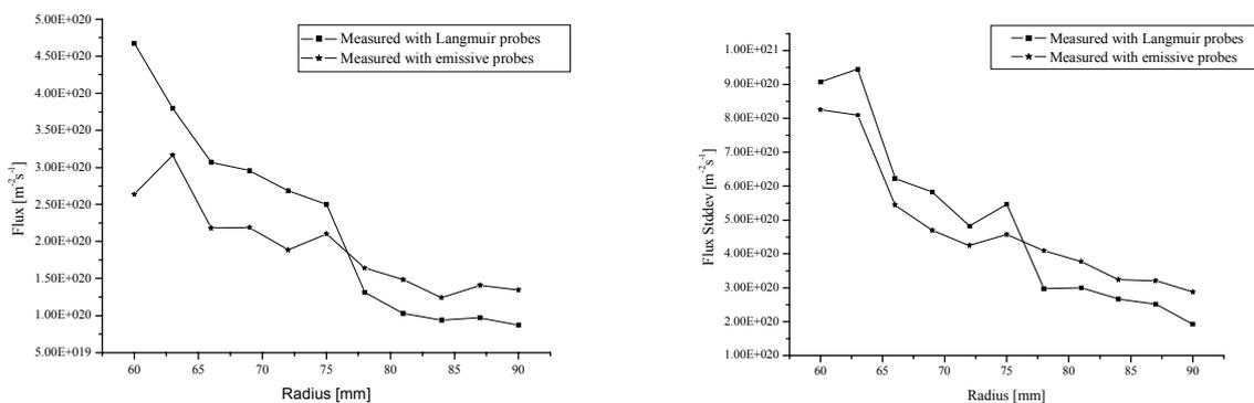
Fig. 4: Radial profile of the fluctuation-induced flux; (a) average values; (b) rms-values; in both cases the emissive probes have been once not heated ("Langmuir probes") and heated to electron emission.
