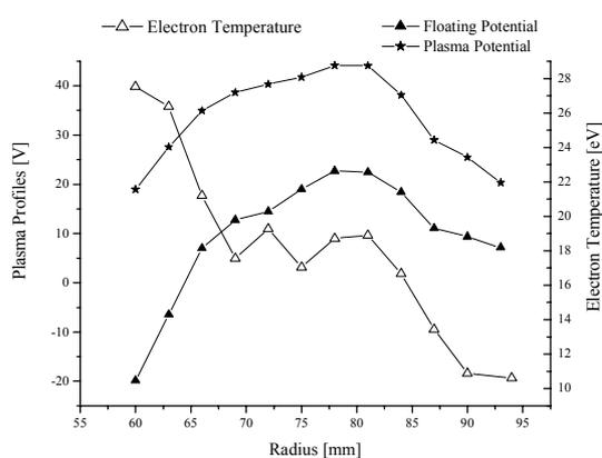
Fig. 2: The plasma and floating potential profile. The electron temperature profile was calculated choosing  $\mu = 2.04$ .
