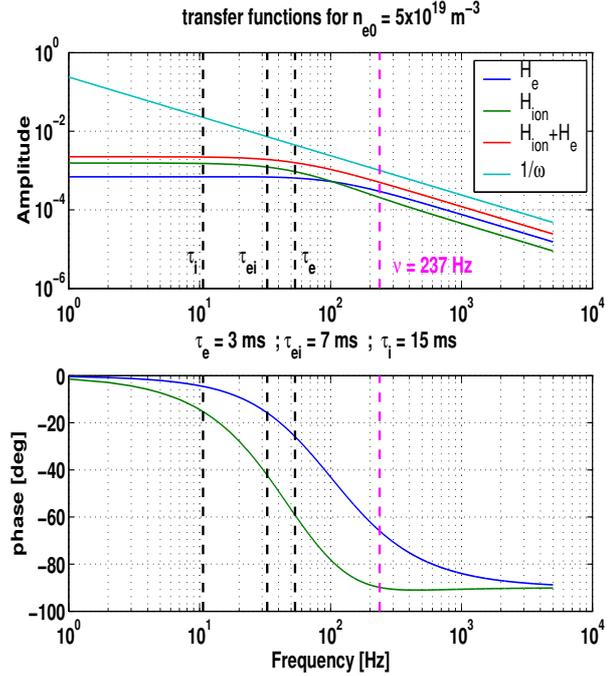
Figure 3 : The phase and amplitude of the transfer function calculated with a  $Z_{eff} = 2$  and an ECH power of 1 MW.  $Z_{eff} = 2$  means that the ionic density is equal to 70 % of the electron density
