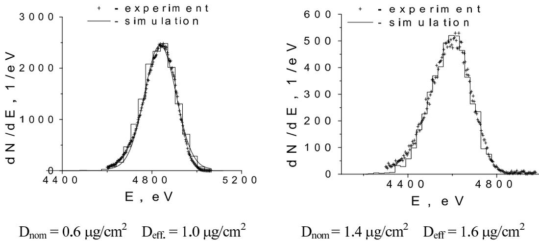
**Fig.1** Energy spectrum of  $\text{H}^+$  ions with  $E_0 = 5040 \text{ eV}$  transmitted through DLC different foils
