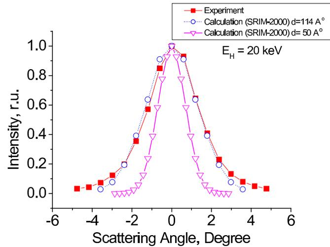
**Fig.4** Angle distribution of  $H^+$  ions transmitting through the foils
