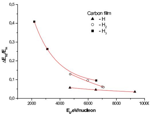
**Fig.2** Energy resolution of diamond-like film with  $D_{\text{nom}} = 30 \text{ \AA}$  ( $0,6 \mu\text{g}/\text{cm}^2$ )
