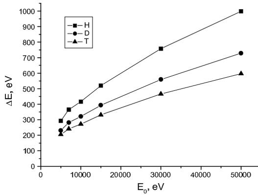
**Fig.3** Energy dependence of ion straggling in the  $6 \mu\text{g}/\text{cm}^2$  foil for different ions
