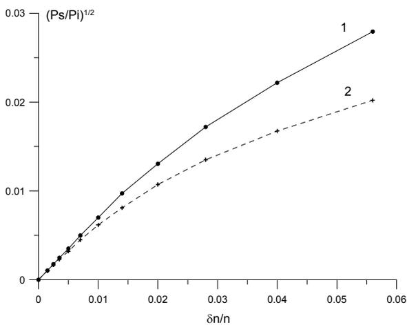
Fig. 1. Scattering signal versus oscillations amplitude.  $n_{e0} = 10^{13} \text{ cm}^{-3}$ ,  $f = 9 \text{ GHz}$ ,  $B_0 = 60 \text{ mT}$ ,  $\lambda_{\text{fluct}} = 2 \text{ mm}$ , horn  $5.6 \times 3.4 \text{ cm}^2$ . Curve 1 —  $\delta n/n > 0$ , 2 —  $\delta n/n < 0$  at the UHR.
