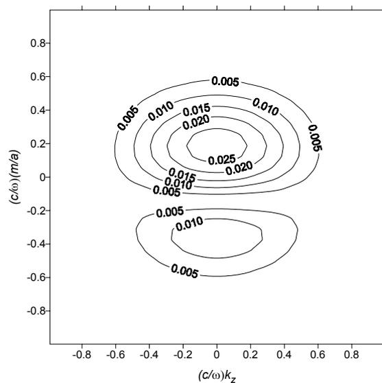
Fig. 3. Topological map of  $|C|$  distribution for the horn  $5.6 \times 3.4 \text{ cm}^2$ . Other parameters are the same.
