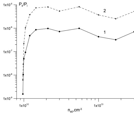
Fig. 2. Dependence of the scattering signal on the central density.  $\delta n/n = 0.5\%$ , other parameters are the same. Curve 1 — horn  $2.3 \times 1.0 \text{ cm}^2$ , 2 — horn  $4.0 \times 2.2 \text{ cm}^2$
