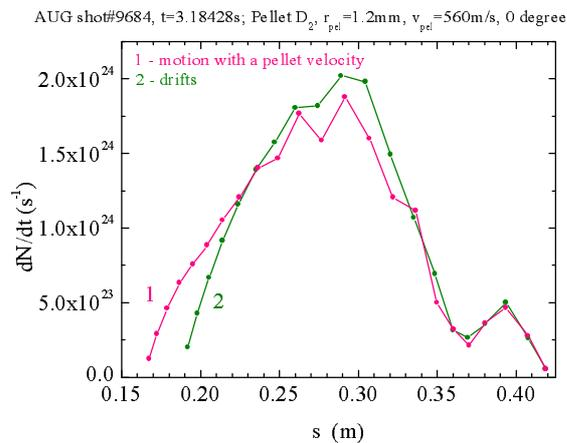
Figure 4. Ablation profiles for alternatives a) and b).
