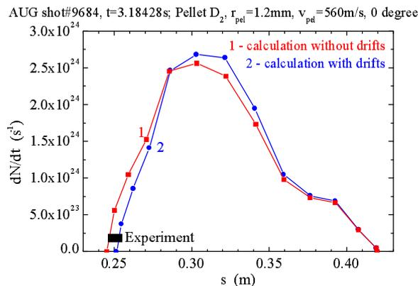
Figure 2. Ablation rate variation along the pellet path for the cases with and without drift.
