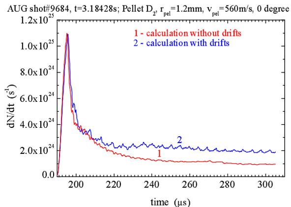
Figure 3. Self-consistent value of ablation rate in a representative flux tube.
