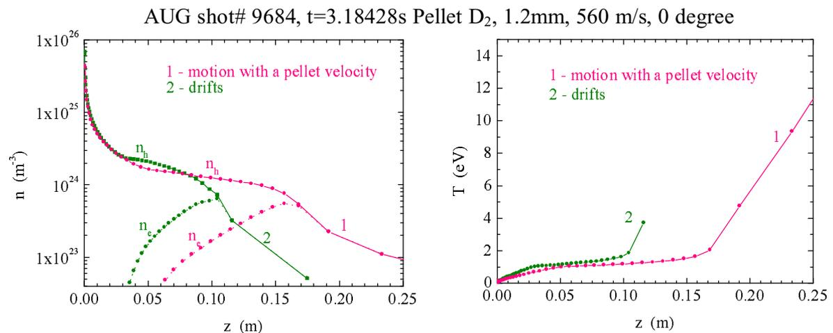
Figure 5. Density (left) and temperature (right) profiles along magnetic field lines at the point of ablation rate maximum (see also Fig. 4) without drift (pink lines) and with drift (olive lines).
