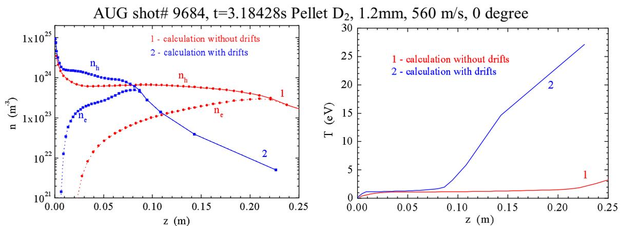
Figure 1. Density (left) and temperature (right) profiles along magnetic field lines at the point of ablation rate maximum (see Fig. 2) without drift (red lines) and with drift (blue lines). It should be noted that in the case without drift cloud propagates up to 6 meters, but only inner region is shown to provide a comparison with calculation with drift.
