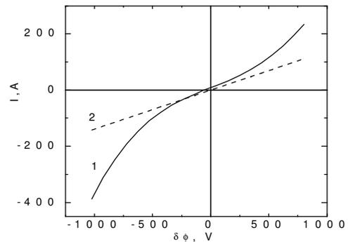
Fig.7. I-V characteristic for  $\kappa < 1$ : 1-calculated characteristic; 2-theoretical prediction.
