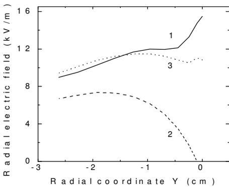
Fig.3. Radial electric field profile for  $\kappa > 1$ : 1- calculated profile; 2- theoretical prediction for  $V_{||} = 0$  at the separatrix; 3- theoretical profile for the code boundary condition.
