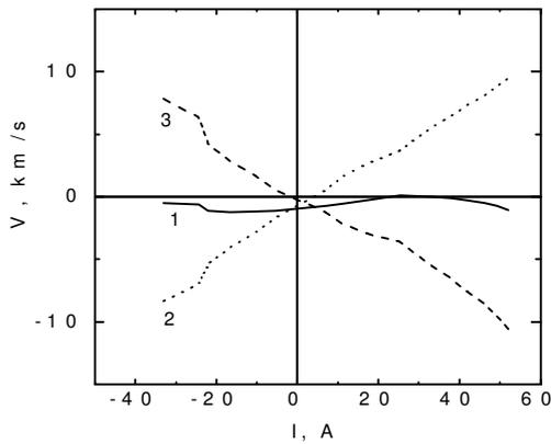
Fig.2. Dependencies of the different components of averaged poloidal velocity on the net current for  $\kappa > 1$ : 1- net poloidal velocity; 2-  $\vec{E} \times \vec{B}$  velocity; 3- poloidal projection of the parallel velocity.
