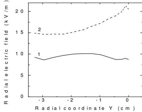
Fig.6. Radial electric field profile for  $\kappa < 1$ : 1- calculated profile; 2-theoretical prediction.
