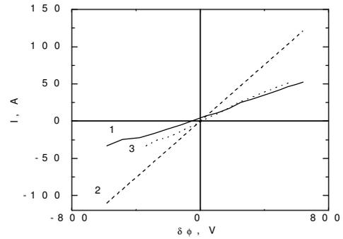
Fig.4. I-V characteristic for  $\kappa > 1$ : 1-calculated characteristic; 2-theoretical prediction for  $V_{||} = 0$  at the separatrix; 3-theoretical characteristic for the code boundary condition.
