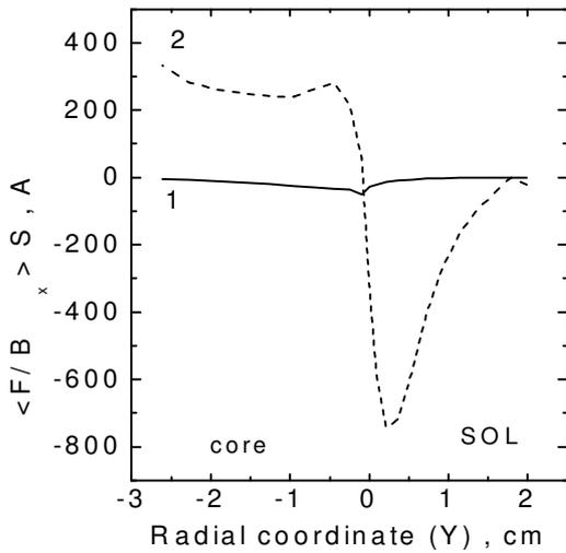
Fig.1. Toroidal components of the averaged momentum balance for discharge parameters  $\phi|_{electrode} = 1000 V$ ,  $n|_{-1cm} = 2 \cdot 10^{19} m^{-3}$ ,  $T_i|_{-1cm} = 40 eV$ : 1- ion-neutral friction force; 2- divergence of the radial flux of toroidal momentum.
