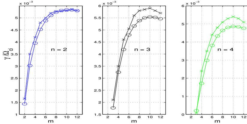
Figure 2: ITG growth rates: values obtained with the SL code ( $\times$ ) and with LORB5 ( $o$ ).
