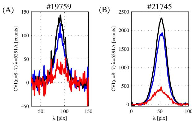
Figure 2. C/X C/I(n=8→7) lines @ 5291Å ( $\bar{n}_e \sim 3.10^{19} \text{m}^{-3}$ ). The photon collection has been enhanced by ~20x, corresponding to an increase of S/N ratio by ~5x.
