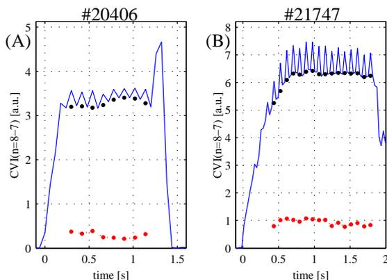
Figure 1. C/X C/I(n=8→7) line ( $\lambda=5291\text{\AA}$ ) intensity for two ohmic shots with  $\bar{n}_e \sim 6.10^{19} \text{m}^{-3}$ . Dots represent interpolated passive and calculated active intensities. (A) Before DNBI upgrade: A/P~12%. (B) After upgrade: A/P~20%.
