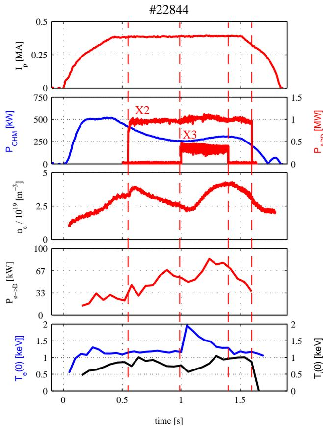
Figure 4. Discharge #22844 has been pre-heated with X2 ECR off-axis heating, before vertical injection of X3 at 1s.  $T_e(0)$  rises of ~80% at the X3 injection whereas  $T_i(0)$  decreases of 30% following the ion heating power ( $P_{ei}$ ) evolution. After injection both temperatures relax on the same time scale as the density increase.
