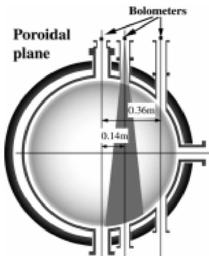
Figure 1. Experimental setup. Three housing metal foil bolometers are installed on the vertical ports
