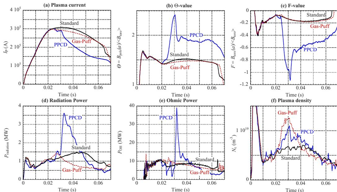
Figure 3. Typical waveforms of plasma current  $I_p$ , reversal parameters  $\Theta = B_{\text{polo}}(a)/\langle B_{\text{toro}} \rangle$  and  $F = B_{\text{toro}}(a)/\langle B_{\text{toro}} \rangle$ , total radiation power  $P_{\text{rad}}$  and Ohmic power  $P_{\text{OH}}$ .
