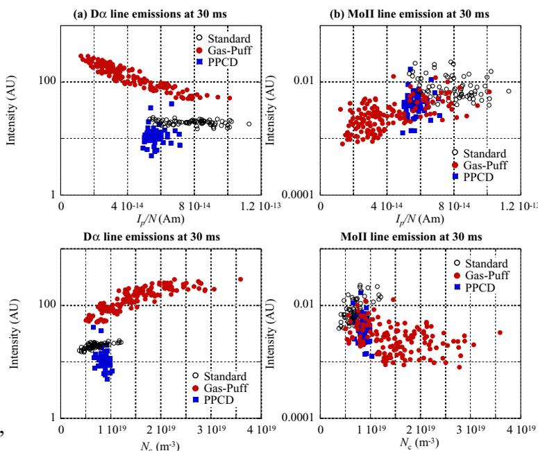
Figure 5. D $\alpha$  line and impurity lines emissions in standard, gas puffing, and PPCD discharge at 30ms. (a); Da line 6561Å. (b); MoII line 3272Å.
