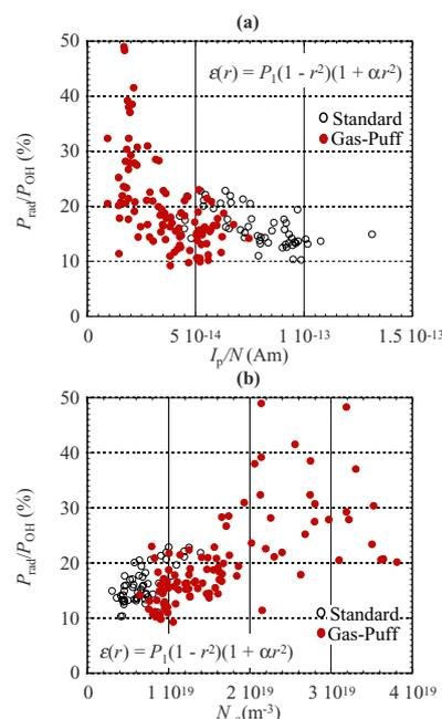
Figure 4. Radiation fraction.
