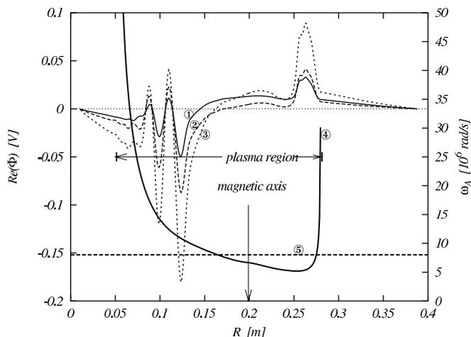
Fig.2 Radial profiles of the solutions  $\Re \Phi$  in the midplane ( $Z = 0$ ) for the antennas ① — ③ described in the Fig.1. Also shown (in the lower part of the graph) are the approximate radial profiles of the Alfvén frequency, ④ and the pump frequency,  $\omega = 8 \cdot 10^6 \text{ rad/s}$ , ⑤.
