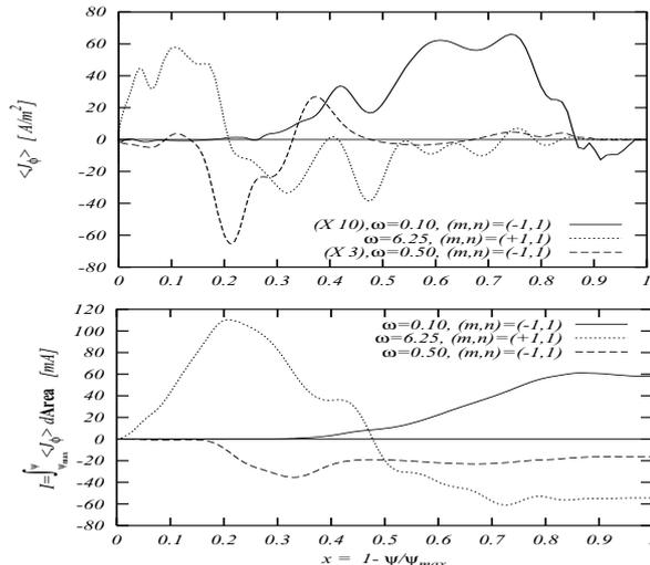
Fig.7  $\psi$ -dependence of the magnetic surface averaged toroidal rf current drive components (top) and of the corresponding integrated current component,  $I(x) \equiv \int_0^x \langle j_\phi \rangle da$  (bottom) for the indicated antenna parameters.
