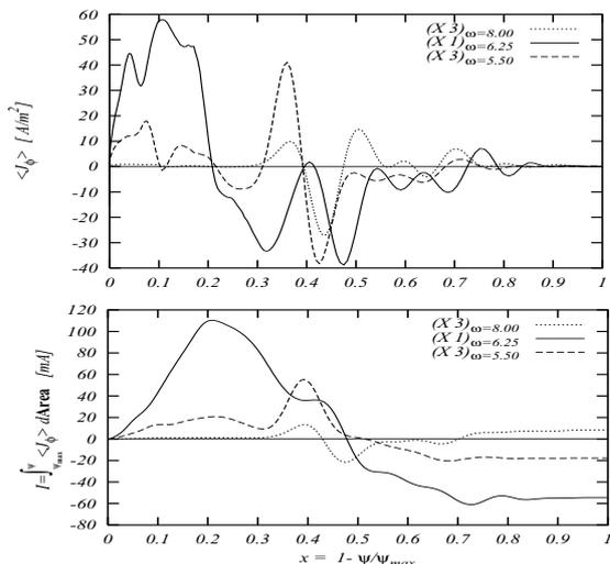
Fig.6 Top: Magnetic surface averaged toroidal current component  $\langle j_\phi \rangle$ , for three wave frequency values, namely,  $\omega/10^6 \text{ rad} \cdot \text{s}^{-1} = 8, 6.25$  and  $5.5$ ; bottom: corresponding integrated toroidal current component,  $I(x) \equiv \int_0^x \langle j_\phi \rangle da$ , with  $da$  — the area element.
