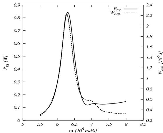
Fig.4 Dependence of the total power deposition and e.m energy on the pump frequency in the range  $5.5 \leq \omega/(10^6 \text{ rad/s}) \leq 8$ ; all other parameter are the same as in the Ref. case.
