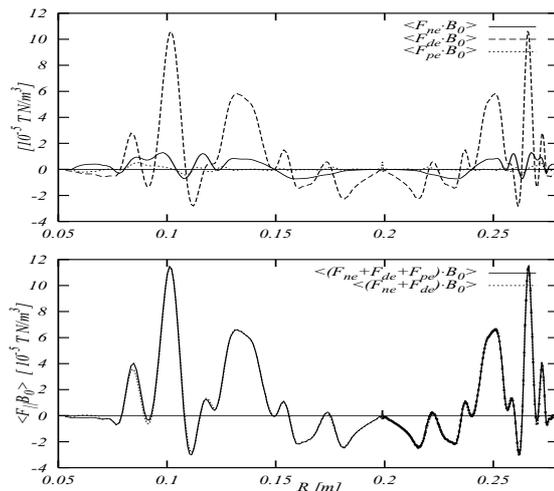
Fig.5 Magnetic surface averaged forces  $\langle F_{e,l} \cdot B_0 \rangle$  ( $l = L, H$  and the force associated with the wave pressure) (top) and  $\langle \Sigma F_{e,l} \cdot B_0 \rangle$  (bottom) corresponding to the pump frequency  $\omega = 6.25 \cdot 10^6 \text{ rad/s}$
