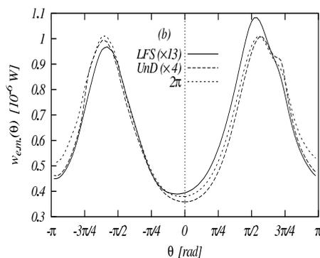
Fig.3 Polar ( $\theta$ ) dependence of the radially integrated local power deposition (top) and of the e.m. energy density (bottom) for the three types of antenna considered in Fig.1 and 2. The solid, dashed and dotted curves correspond, respectively to LFS, UnD and  $2\pi$  circular antennas.
