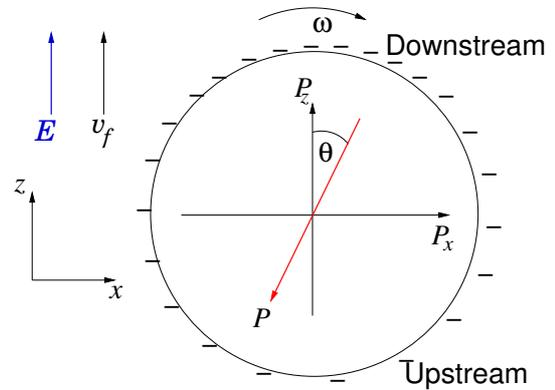
Figure 1: Schematic illustration of the charged sphere and dipole moments.
