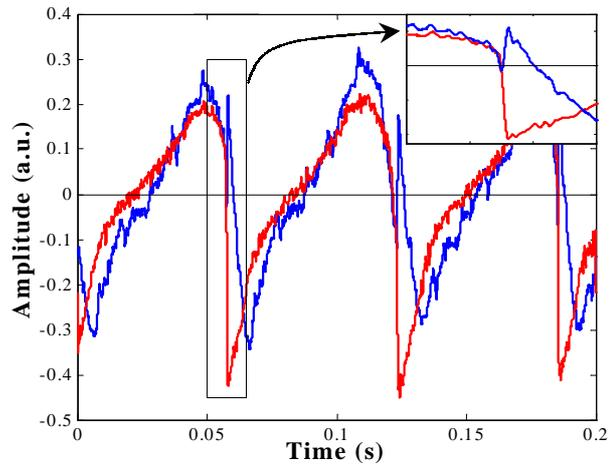
FIG. 4. Discharge current (blue) and total plasma light inside the void (red)
