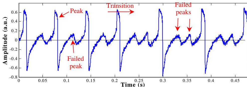
FIG. 5. Transition (between 1 and 2 failed peaks) appearing before the heartbeat instability stops.
