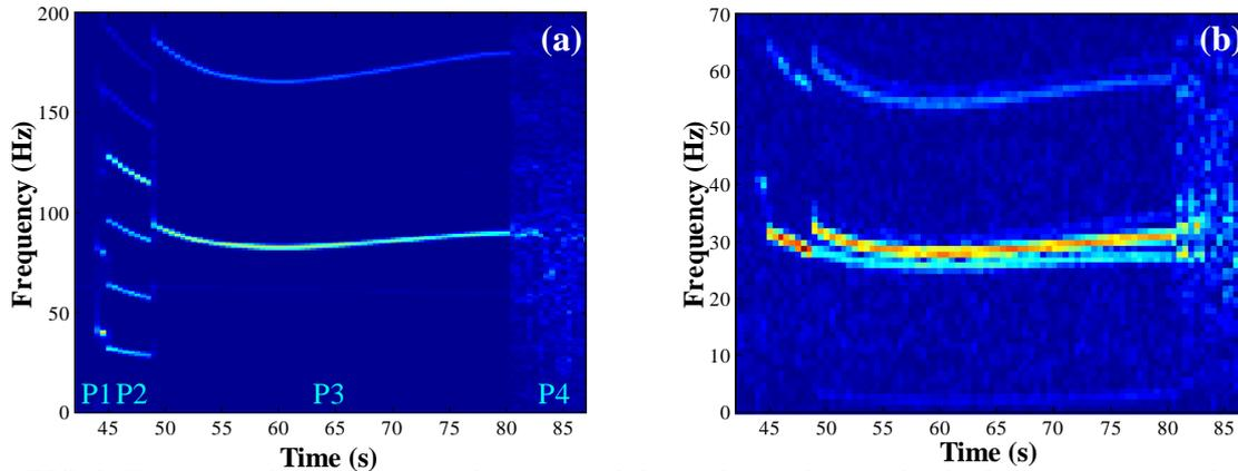
FIG. 3. Fourier analysis of the growth start instabilities observed (a) in the discharge current amplitude (b) in the optical signal recorded near the plasma edge
