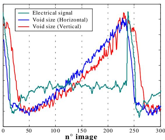
FIG. 6. Electrical signal and void size evolution
