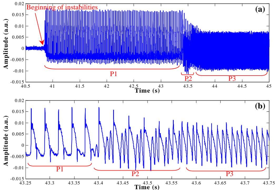
**FIG. 1.** (a) First phases of the growth start instabilities observed in the discharge current amplitude (b) zoom of (a) on the phase transitions
