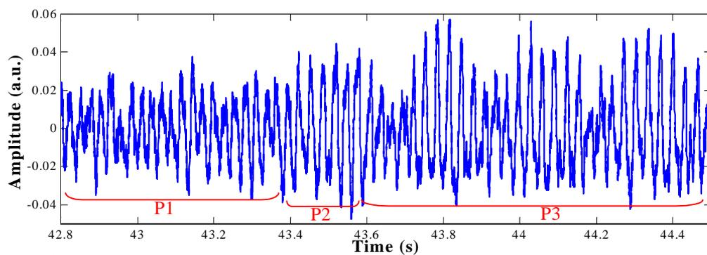
**FIG. 2.** First phases of the growth start instabilities observed in the near edge plasma light
