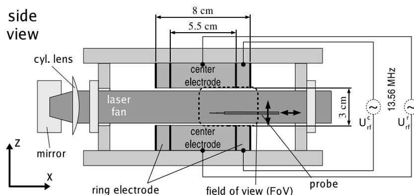
Figure 1: Scheme of the IMPF plasma chamber with the field of view of the camera.
