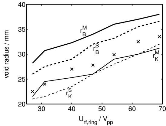
Figure 3: Radial extent of the void as function of the ring electrode voltage  $U_{rf}^r$ . Crosses mark the observed particle positions,  $r_{B,K}^M$  are calculated equilibrium positions from probe measurements, using the Barnes formula and Khrapak's model respectively.  $r_{B,K}^S$  are derived from simulated plasma parameter profiles.
