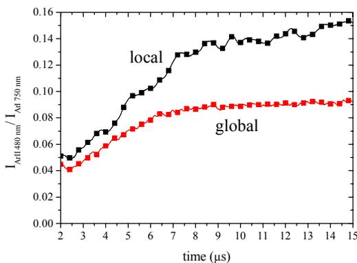
Fig.4a Local (optical fiber probe on axis) and diameter-integrated measurements of ratio of ArII and ArI line intensities in second  $rf$  pulse (delay 40 μs,  $P_{rf} = 1.4$  kW).
