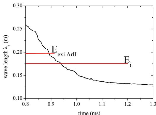
Fig.5a: Variation of the helicon wave length in the beginning of the plasma pulse
