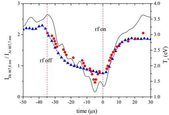
Fig.3b: Ratio of He 667,8 nm and Ar 667,7 nm line intensities and electron temperature in the afterglow and the second pulse.
