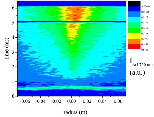
Fig.1b: local intensity of ArI 750 nm line in the main and second pulse ( $B = 40.5$  mT,  $P = 0.6$  Pa, delay  $40 \mu\text{s}$ ,  $P_{rf} = 1.4$  kW)
