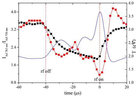
Fig.3a: Ratio of Ar 763 nm and Ar 750 nm line intensities and electron temperature in the afterglow and the second pulse; for comparison,  $T_e$  from probe measurements.
