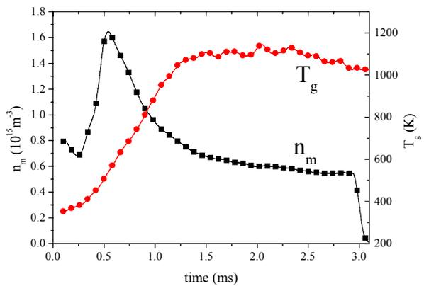
Fig.2b:  $^3P_0$  density and gas temperature determined from Doppler absorption profile ( $B = 40.5$  mT,  $P = 0,3$  Pa,  $L = 1.4$  kW)
