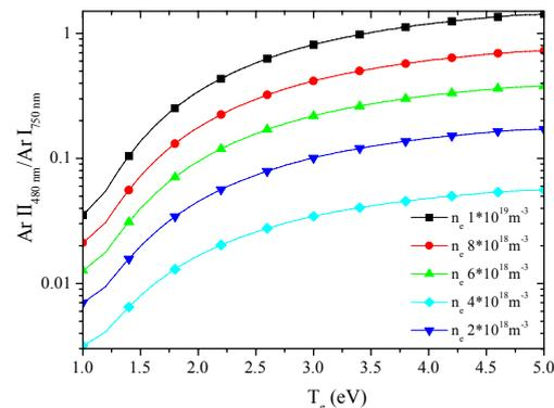
Fig.4b: Calculated Ratio of of ArII 480,6 nm and ArI 750,4 nm line intensities ( $T_g = 1000$ K,  $P = 0.3$  Pa).
