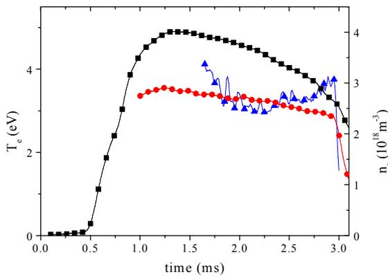
Fig.2a: Electron density and electron temperature determined from metastable density ( $^3P_0$  niveau)
