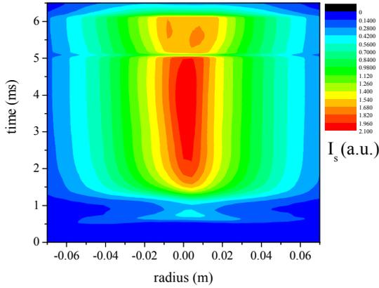
Fig.1a: local measurements of ion saturation current in the main and second pulse over the radius 0.5 m from the antenna centre
