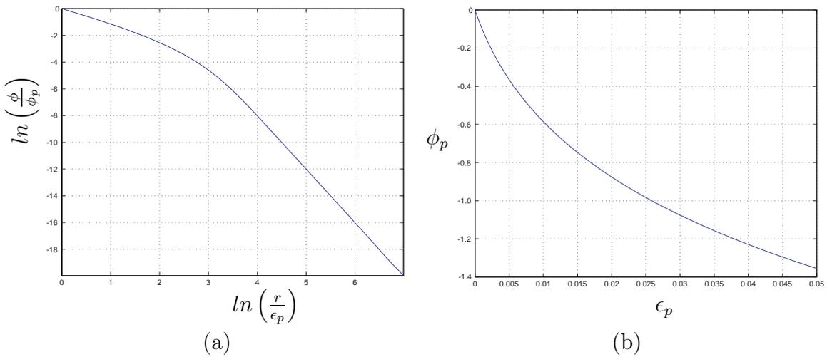
FIGURE 2: Plots of (a) potential profile and (b) dust floating potential vs.dust size for Argon.
