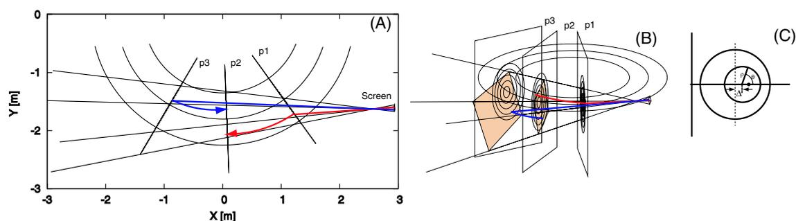
Fig.1: Geometry of the tangentially viewing camera system. On the equatorial plane (A) and the bird-view diagram (B) are shown. To project images on the plane (p2) we assume a magnetic flux shifted by  $\Delta(\rho) = \Delta_0(1 - \rho^2)$  shown in (C).
