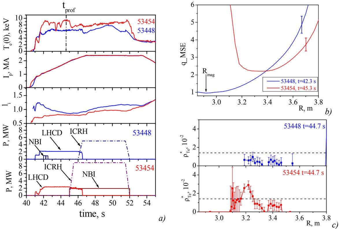
Fig. 1. Comparison of two similar shots with (53454) and without (53448) eITB formation: a) temporal evolution of central electron temperature ( $T_e$ ), internal inductance ( $l_i$ ), and heating power; b) differences in  $q$  profile behaviour measured by MSE diagnostic; c)  $\rho_{Te}^*$  profiles at the time marked as  $t_{prof}$  (Fig. 1,a) in comparison with the critical value determining ITB existence (dashed lines).
