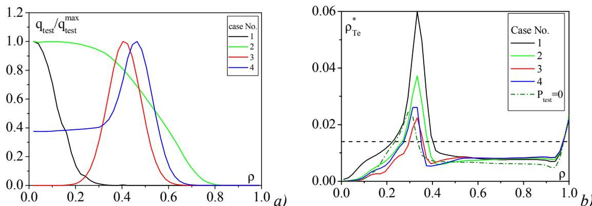
Fig.3. a) Normalised profiles of test heating power,  $q_{test}$ ; numbers are used as a markers of calculation run; b)  $\rho_{Te}^*$  values for calculated electron temperature profiles.
