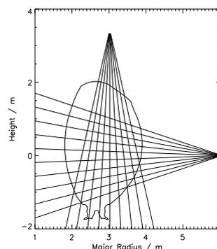
Figure 1: Lines of sight of the JET neutron profile monitor.
