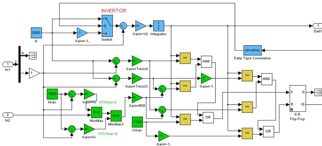
Fig. 2. Simulink-subsystem of the actuator.
