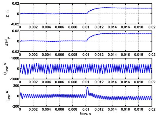
Fig. 6. Time trajectories of the plasma vertical position, voltage and current in HFC.
