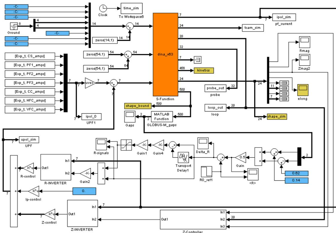
Fig. 4. General scheme for Simulink model developed for GLOBUS-M device.
