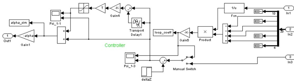
Fig. 3. Simulink subsystem for Z-controller simulation.
