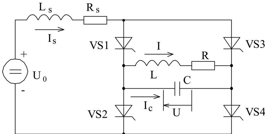
Fig. 1. The electrical scheme of one phase bridge current inverter.
