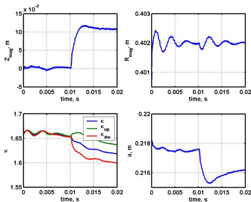
Fig. 5. Time trajectories of the vertical and radial plasma positions, elongation and minor radius.
