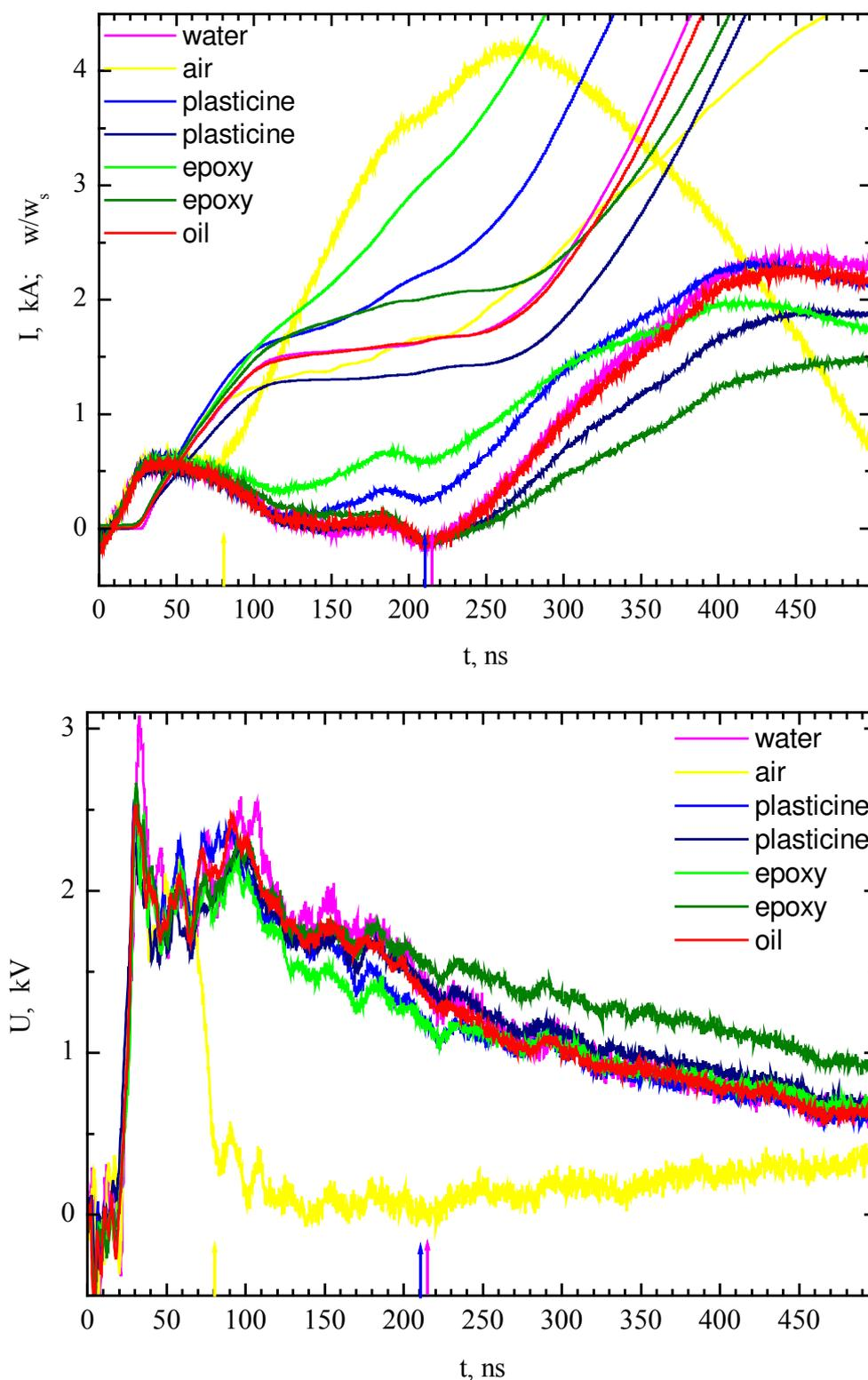
Fig.2. The deposited energy, heating current and voltage at the explosion of  $25 \mu\text{m}$  tungsten wires ( $l = 12 \text{ mm}$ ,  $L = 570 \text{ nH}$ ) submerged into different media.  $w_s$  – sublimation energy. Arrows denote the moment of breakdown.
