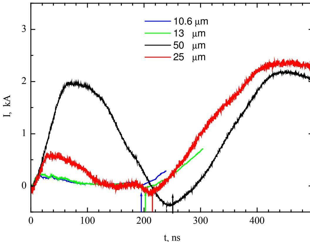
Fig.3. The current at the explosion of tungsten wires ( $l = 12$  mm,  $L = 570$  nH) submerged into water. Arrows denote the moment of breakdown.
