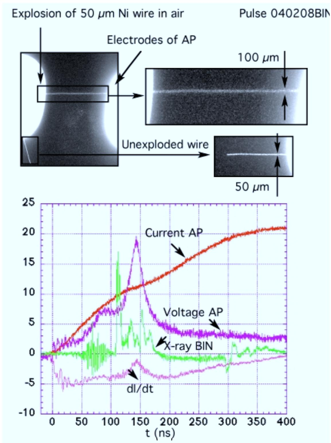
Fig. 1. X-ray radiograph of 50  $\mu\text{m}$  Ni wire in open air and current, voltage,  $di/dt$  and X-ray signals (arbitrary units).
