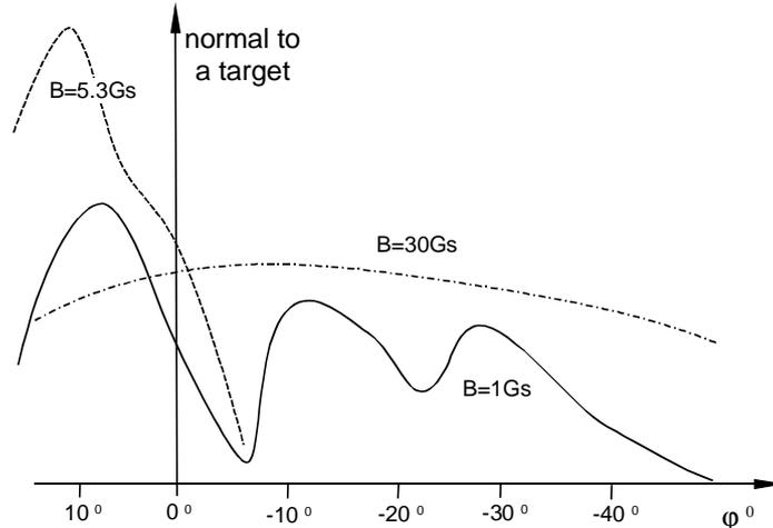
**Fig. 4b** The angular distribution of the spreading laser plasma at a range of  $R=6$  cm from the target.
