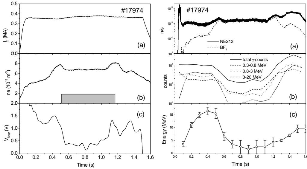
Figure 2: **Left:** Time evolution of plasma current, central line averaged density and loop voltage for deuterium discharge 17974. The shaded area shows the time interval for LH injection; **Right:** For the same pulse: Time traces of  $BF_3$  and NE213 scintillator, photon counts detected by the gamma-ray system, and maximum measured gamma energy.
