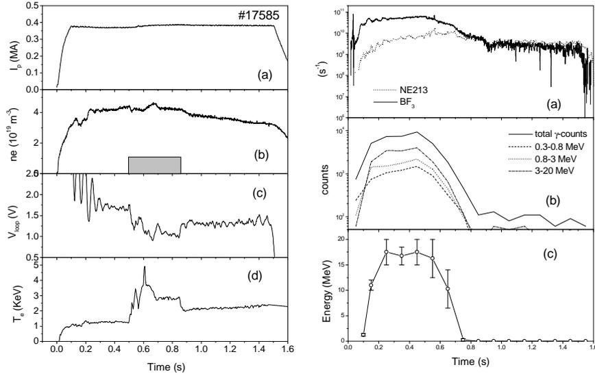
Figure 1: **Left:** Time evolution of plasma current, central line averaged density, loop voltage, and electron temperature at plasma axis for deuterium discharge 17585. The shaded area shows the time interval for ECRH heating; **Right:** For the same discharge: Time traces of  $BF_3$  and NE213 scintillator, photon counts detected by the gamma-ray system (total and in several energy ranges), and maximum measured gamma energy.
