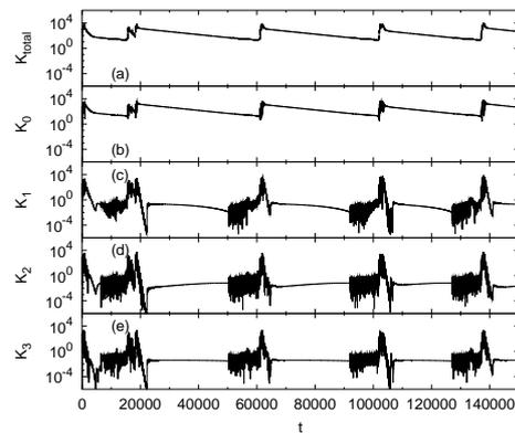
Figure 1: Time evolution of (a) total kinetic energy and kinetic energy of (b) sheared flows  $K_0$ , (c) the 1st harmonics  $K_1$ , (d) the 2nd harmonics  $K_2$  and (e) the 3rd harmonics  $K_3$  for  $K_i = 5$ .
