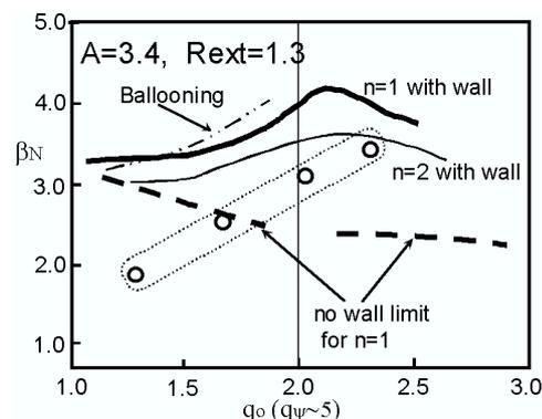
Fig.1 MHD equilibria for the basic operation stage. The reference operation points are shown by circles.
