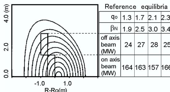
Fig. 2 Beam powers for the reference equilibria shown in Fig. 1, where  $E_b=1.5\text{MeV}$ .
