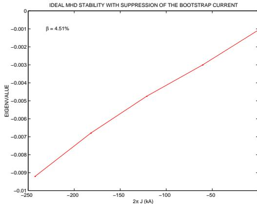
Fig. 3. The unstable eigenvalue of a global external kink mode dominated by the  $m/n = 1/1$  component as function of the toroidal current as the magnitude of the BC is artificially suppressed while keeping its profile fixed.
