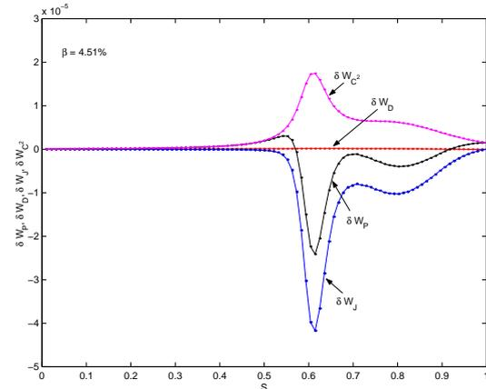
Fig. 4. The radial profiles of energy principle components  $\delta W_{C^2}$ ,  $\delta W_D$ ,  $\delta W_P$  and  $\delta W_J$  for the full ( $-303 kA$ ) selfconsistent BC case at  $\langle \beta \rangle \simeq 4.5\%$  in a 4-period Helias reactor.
