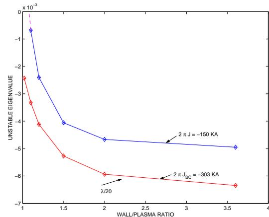
Fig. 10. The unstable eigenvalue  $\lambda$  of a global external kink mode in 4-period Helias reactor equilibria at  $\langle \beta \rangle \simeq 4.5\%$  with a selfconsistent bootstrap current ( $-303kA$ ) and with a model toroidal current of  $-150kA$ .
