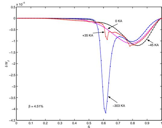
Fig. 8. The contribution of the parallel current drive  $\delta W_J$  to the perturbed energy at  $\langle \beta \rangle \simeq 4.5\%$  for model current profiles of  $-45kA$  and  $+35kA$ , for the selfconsistent BC case ( $-303kA$ ) and for vanishing current.
