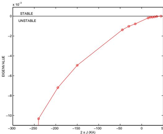
Fig. 7. The unstable global ideal MHD eigenvalue as a function of the toroidal current in a 4-period Helias reactor at  $\langle \beta \rangle \simeq 4.5\%$  for a model current profile that combine the vbootstrap current with counter ECCD.
