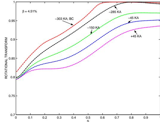
Fig. 6. The  $\iota$ -profiles corresponding to the toroidal current and current profiles of Fig. 5 at  $\langle \beta \rangle \simeq 4.5\%$ . For reference, the profile of the selfconsistent BC ( $-303kA$ ) case is also shown.
