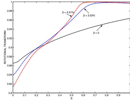
Fig. 2. The rotational transform  $t$ -profiles in vacuum, at  $\langle \beta \rangle \simeq 3\%$  and at  $\langle \beta \rangle \simeq 4.5\%$  obtained with converged selfconsistent bootstrap currents in the collisionless  $1/\nu$  regime in a 4-period Helias reactor.
