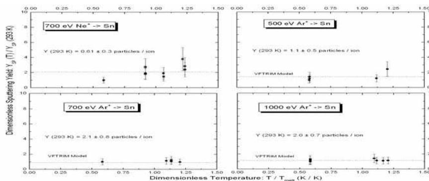
Figure 2: Experimental results for heavy-ion bombardment of tin at 45° incidence. Also shown is the dimensionless sputtering yield found using VFTRIM<sup>18</sup>.
