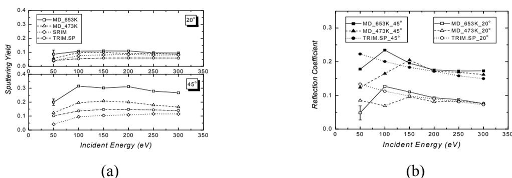
Figure 1. (a) The sputtering yield as the function of incident energy, and (b) The reflection coefficient as the function of incident energy. The error bars shown are representative of the statistical error for every point.
