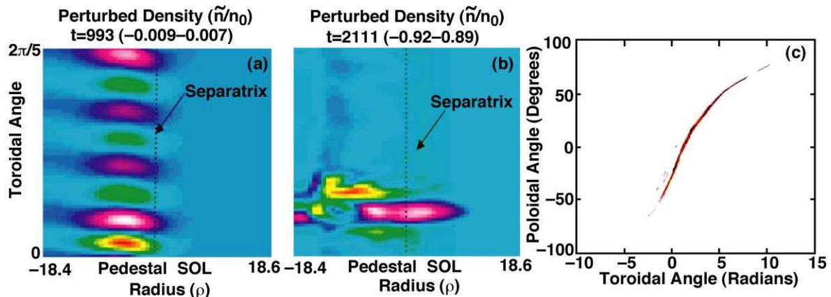
Fig. 3 (a) Density perturbation from nonlinear simulations at early times shows the expected peeling-ballooning structure (here  $n=20$ ) in the pedestal region. (b) Later a fast radial burst across the separatrix occurs, localized toroidally, but extended along the field as shown in (c).
