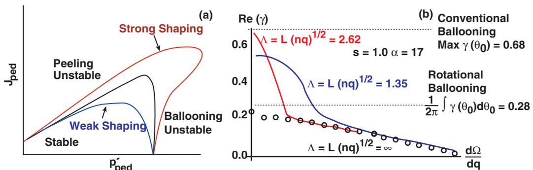
Fig. 1. (a) Schematic diagram of peeling-ballooning stability bounds vs. edge current and pressure gradient for different shaped equilibria. (b) Growth rate vs flow shear for  $n \rightarrow \infty$  (circles) and for two finite values of  $n$ .
