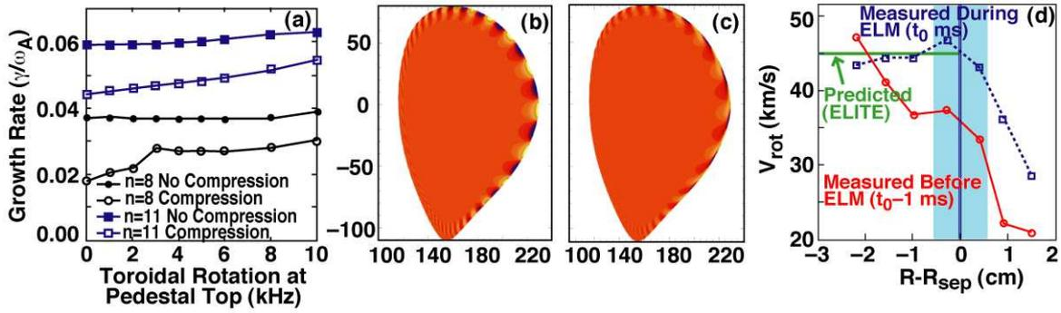
Fig. 2. (a) Growth rate vs. pedestal flow, and  $n=11$  mode structure for (b) no flow and (c)  $\Omega_{\text{ped}} = 10$  kHz. (d) Measured rotation profile before and during an ELM. The measured rotation during an ELM is compared to the calculated mode rotation using pre-ELM profiles.
