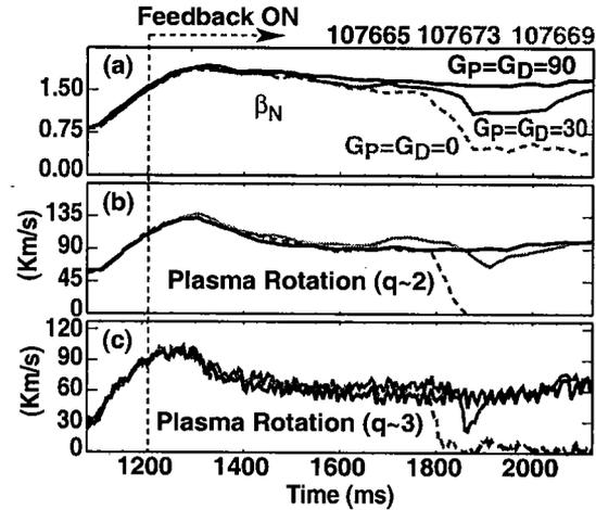
Fig. 1. Low rotation plasma target for RWM feedback studies produced using mostly perpendicular neutral beam sources. (a) Feedback gain scan and its effect on  $\beta_N$ . (b,c) Absence of correlation between feedback gain and plasma rotation suggests direct feedback stabilization of the RWM.
