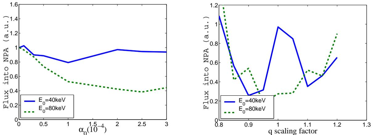
FIG. 2: Results of NPA signal flux modeling for two energies  $E_{b0} = 80keV$  and  $40keV$  used at the start of numerical runs. The modeled fluxes are shown as functions of mode amplitude  $\alpha_0$  (left) and the scaling factor for the safety factor profile (right).
