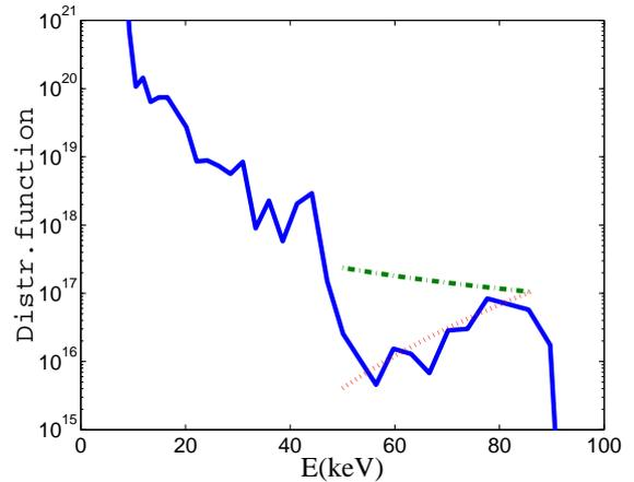
FIG. 1: NPA signal spectrum for shot #108730 at  $t = 400msec$  (solid curve) and its approximation at high energies by the slowing down distribution without loss (dash-dotted line) and with finite loss time, Eq.(2) (dotted line).
