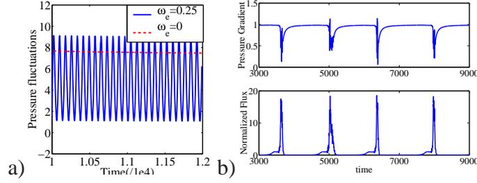
Figure 1: a) Time evolution of the pressure fluctuations  $\sqrt{\int \tilde{p}^2}$  with and without frozen shear flow b) Time evolution of pressure gradient  $[|\partial_r \tilde{p}| / (\Gamma_{tot} / \chi_{\perp})]$  and turbulent flux  $[2\gamma_0 |\tilde{p}|^2 / \Gamma_{tot}]$  at the barrier center observed from the 1D model (3-4)
