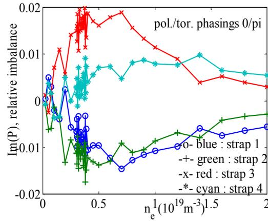
**Figure 3** :  $n_e$  scan, imbalance on reactive power for phasing  $(\phi_p, \phi_t) = (0/\pi)$ . Strap numbering as fig. 1.
