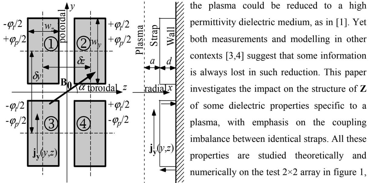
**Figure 1** : sketch of the test antenna studied in this paper. For numerical scan,  $w_z=0.147m$ ,  $w_y=0.264m$ ,  $\delta y=0.36m$ ,  $\delta z=0.28m$ ,  $a=5cm$ ,  $d=16.5cm$ . RF frequency 48MHz,  $B_0=2.41T$ , pitch angle  $\alpha=7^\circ$ .
