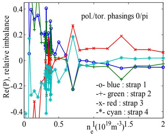
**Figure 2** :  $n_e$  scan, imbalance on active RF power for phasing  $(\phi_p, \phi_t) = (0/\pi)$ . Strap numbering as fig. 1
