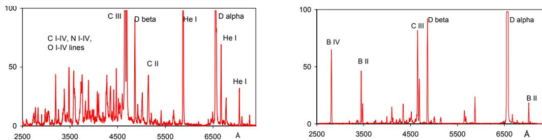
Fig.4 OMA Spectra in Globus-M discharge before (left) and after boronization (right)
