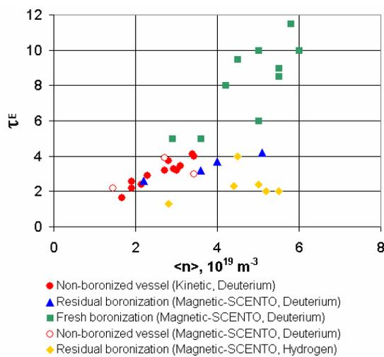
*Fig.3 Energy confinement time in boronized and non boronized vessel versus average density*
