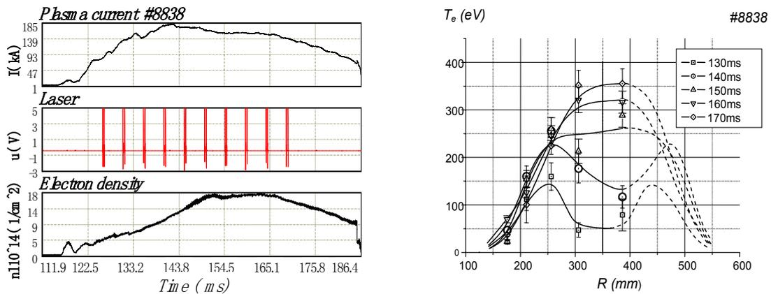
Fig. 1 Plasma current, laser pulse train and line integrated density (left). Electron temperature profile variation (right) in discharge #8838
