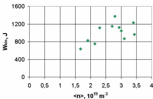
Fig.2 Plasma energy content (kinetic) versus average plasma density in OH deuterium discharge.
