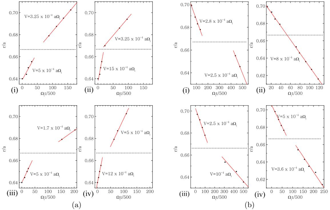
Figure 3: Propagation velocity for (a) positive pulses and (b) negative pulses. Amplitudes ( $A$ ) relative to the local density and width ( $W$ ) relative to  $a$  are: (i)  $A = 0.05$ ,  $W = 0.0005$ ; (ii)  $A = 0.1$ ,  $W = 0.0005$ ; (iii)  $A = 0.05$ ,  $W = 0.001$ ; (iv)  $A = 0.1$ ,  $W = 0.001$ .
