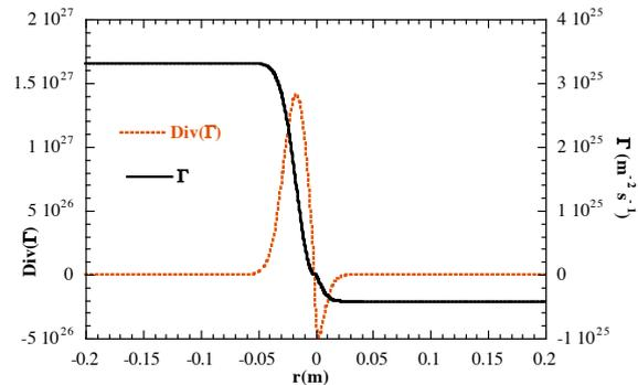
Figure 2. ECH-induced electron flux and its divergence
