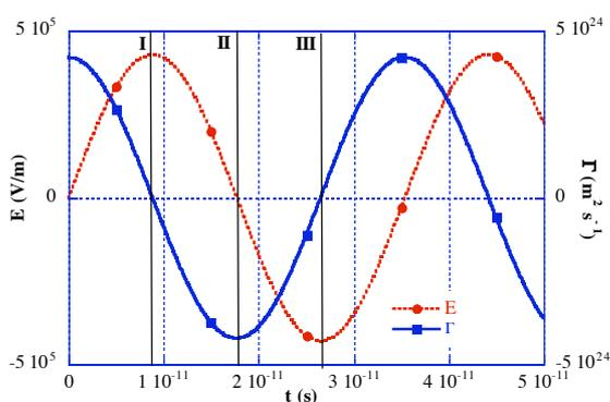
Figure 3. Time evolution of flux and electric field for  $r=0.02$  m.
