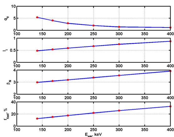
Fig. 3. The dependence of safety factor  $q_0$ , internal inductance  $l_i$ , normalized beta  $\beta_N$  and portion of fast ion  $f_{fast}$  on energy  $E_{NB}$  of particles injected in plasma
