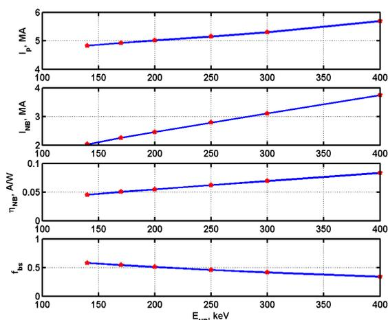
Fig. 2. The dependence of plasma current  $I_p$ , current drive  $I_{NB}$ , efficiency  $\eta_{CD}$ , portion of bootstrap current  $f_{bs}$  on energy  $E_{NB}$  of particles injected in plasma
