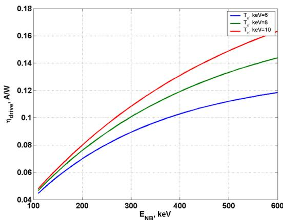
Fig. 1. The efficiency  $\eta_{CD}$  on particle energy  $E_{NB}$
