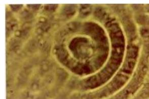
Figure 4 : Diffraction pattern and laser induced periodic structure on CR-39.
