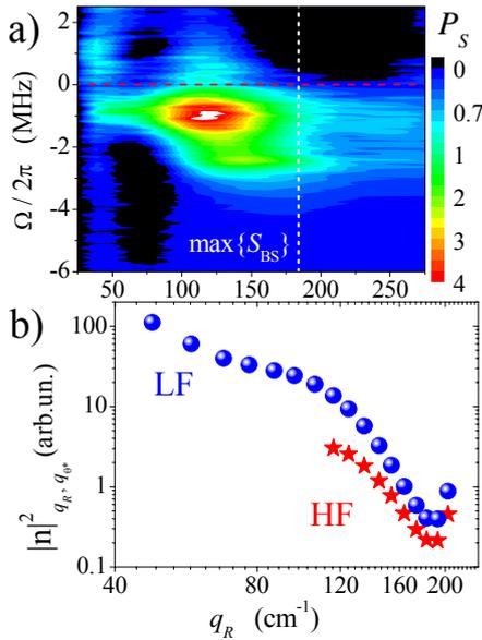
Fig. 7. UHR BS signal spectrum (a) and turbulence wave number spectrum (b) for 32 kA, 64.4 GHz ( $r_{UH} = 5.6$  cm).
