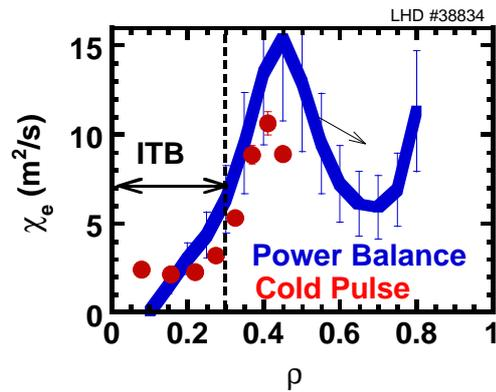
Fig.1 Radial profile of thermal diffusivity estimated from cold pulse and steady state power balance analysis
