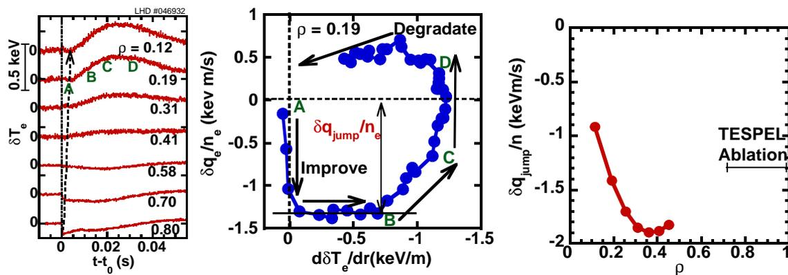
Fig.2 (a) Time evolution of electron temperature after the TESPEL injection and (b) heat flux normalized electron density as a function of temperature gradient 0.005-0.05sec after the TESPEL injection at  $\rho = 0.19$  and (c) radial profile of jump of the normalized heat flux.
