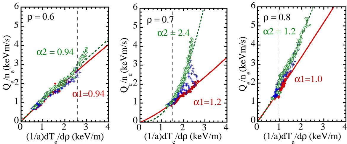
Fig.4 Heat flux normalized electron density as a function of electron temperature gradient 0.06-0.17sec (open circles), 0.17-0.33sec (cross) 0.33-0.57sec (open circles) after the pellet injection at  $\rho = 0.6, 0.7$  and  $0.8$ . The dashed and solid lines are fitting curves with  $Q/n_e = [(1/a)(dT_e/d\rho)]^\alpha$ , where  $\alpha$  is temperature dependence coefficient and before ( $\alpha_1$ ) and after ( $\alpha_2$ ) the phase transition, respectively.
