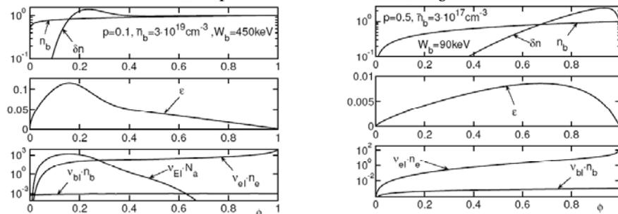
Fig. 2. The profiles of  $n_b$ ,  $\delta n \equiv n_i - n_e$ ,  $\epsilon$ , and the ionization sources along  $\phi$  for high and low beam energy densities, where the electric field ionization is- and is not- important
