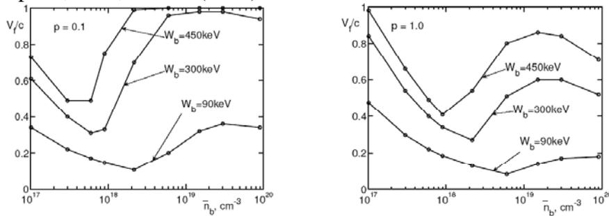
Fig. 1. The front velocity  $V_f$  versus beam density  $\bar{n}_b$  for different  $p$  and  $W_b$
