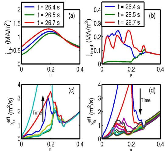
Fig. 5 : Dynamics of various profiles during a GO at  $n_{//} = 1.8$  of shot #33986 (same GO as in Fig. 3). (a) LH current density (deduced from Abel-inversion of the FEB signal, and renormalised using a given current drive efficiency),  $t = 26.4$ ,  $26.5$  and  $26.7$  s. (b) bootstrap current density, same time slices as (a). Effective diffusivities during the decrease (c) and increase (d) phases of the GO, displayed every  $\Delta t = 0.02$  s using the same color code as in Fig. 3.
