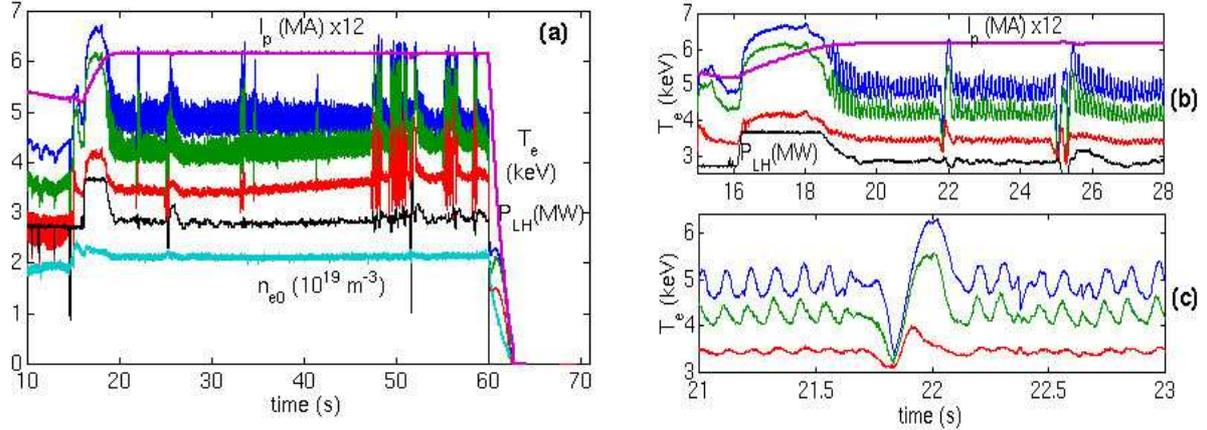
Fig. 1 : Time traces of  $T_e$  (core ECE channels  $r < 0.2$ ), plasma current  $I_p$ , LH power  $PLH$  and central electron density  $n_{e0}$ , shot #33983. In this discharge, the toroidal field decreases slowly from  $B_t = 3.81$  to  $3.76$  T between  $t = 34$  and  $t = 55$  s, which may influence the repetition rate of the GOs.
