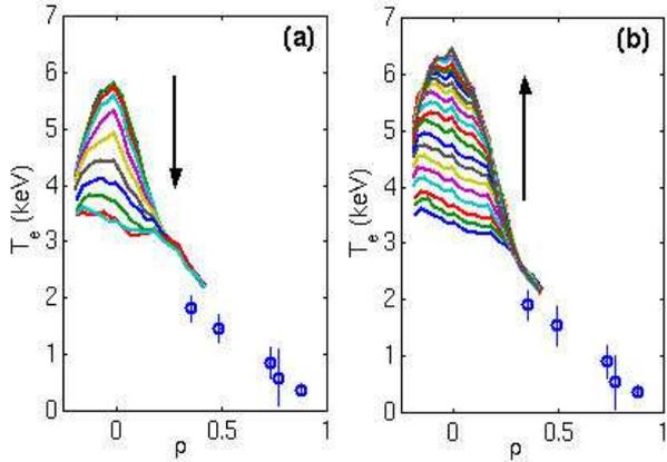
Fig. 3 : Dynamics of  $T_e$  profiles during a GO at  $n// = 1.8$  of shot #33986. (a) slow decrease phase starting from the O-regime level,  $t = 26.4$  to  $26.5$  s; (b) increase phase up to the top of the GO,  $t = 26.5$  to  $26.7$  s. Solid lines correspond to the ECE signal, displayed here every  $\Delta t = 0.01$  s. Blue circles are time-averaged Thomson scattering measurements.
