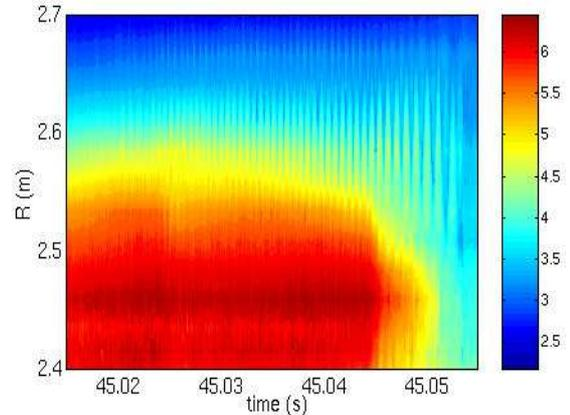
Fig. 4 : Color contour plot of  $T_e$  (keV, fast ECE signal) showing the growth of a multi-resonant ( $m=2, n=1$ ) tearing mode during the fast termination scheme of a GO (shot #33986).
