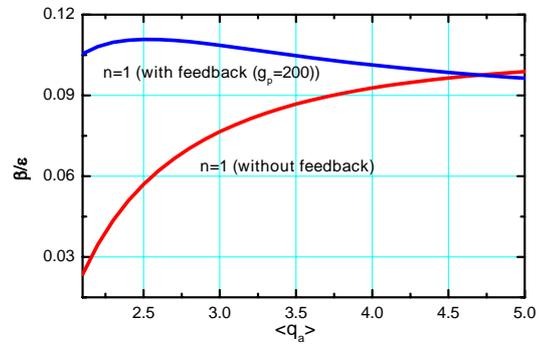
Fig.4. Critical  $\beta/\epsilon$  vs.  $\langle q_a \rangle$
