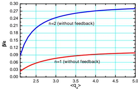
Fig 1. Critical  $\beta$  vs.  $q_a$  for a complete wall.
