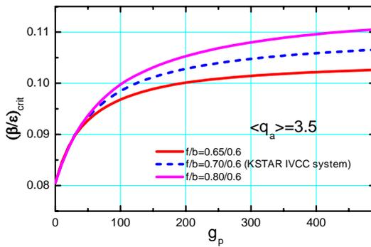
Fig 3. Critical  $\beta/\epsilon$  vs. gain for three different values of feedback coil position.
